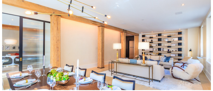
A new chapter: Once the factory floor of an 1883 bookbindery, now occupants live in spaces featuring restored original wood columns and beams. A long-span composite floor system enabled the open design, while assuring low floor vibration and verified superior sound control.
