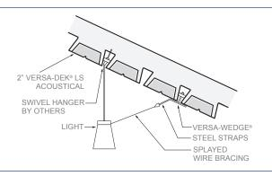
In a sloped application, the Versa-Wedge® system uses a swivel hanger to account for the roof pitch to maintain a crisp aesthetic. Wedge performance is contingent on the placement of the decking to run perpendicular to the slope. For projects requiring ICC approval, the slope cannot exceed 5%.
